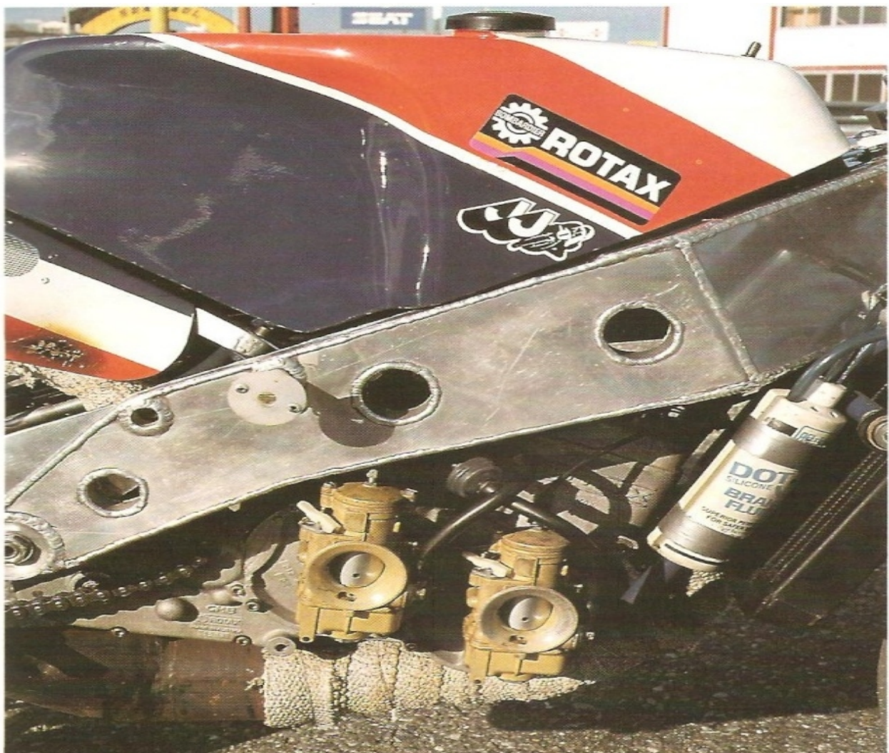
Kobas employs production tandem-twin Rotax rotary-valve engine in seminal twin-spar alloy frame.
